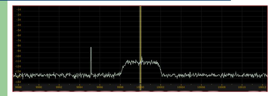
Generator offset 5 kHz below a 10 MHz crystal filter. Filter extends the dynamic range of Perseus SDR receiver Perseus as an FFT spectrum analyzer
