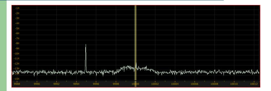
Generator offset 5 kHz below a 10 MHz crystal filter. Filter extends the dynamic range of Perseus SDR receiver
