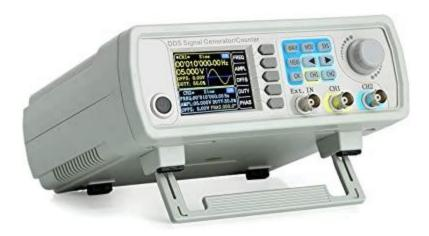
FY6800-60 60 MHz highest frequency Minimum output 1 mV P-P (No dBm calibration) Useless for S meter calibration Amplitude at low levels poor 14 bit DDS uHz frequency resolution Similar model multiple sources No specs for phase noise \$500 eBay
