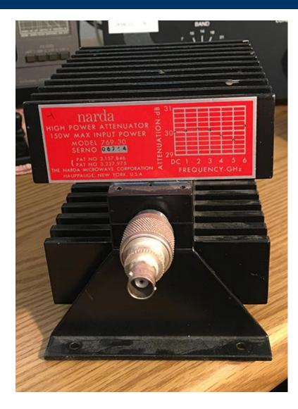
DC to 6 GHz Doubles as a 150 watt dummy load Available: eBay Hamfests QTH.com
