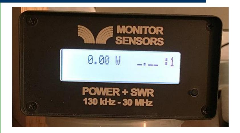
Works on 2200 and 630 meters (136 kHz & 472 kHz)
