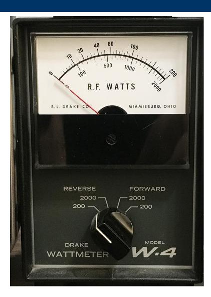
Drake W-4 Used market only No direct SWR reading Removable coupler 200 and 2000 watt scales Reliable Accuracy +/- 10% typical \$200 eBay, HF slugs \$100+
