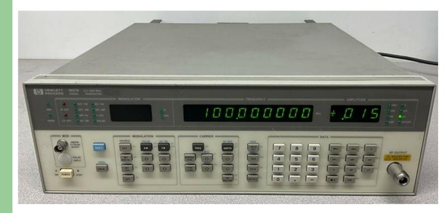
100 kHz to 2.06 GHz, +13 dBm to -143.5 dBm General purpose signal generator
