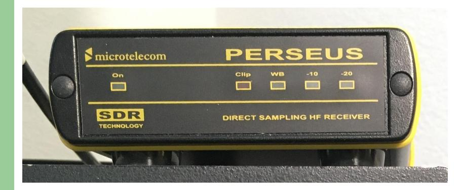
Runs under Windows. 4.1a software recommended SDR tunes to 40 MHz. Also measure TX composite noise Have down-converted 2m, 70cm & 23cm signals to 20 meters. Measured the Icom IC-9700 on all bands Perseus screen capture
