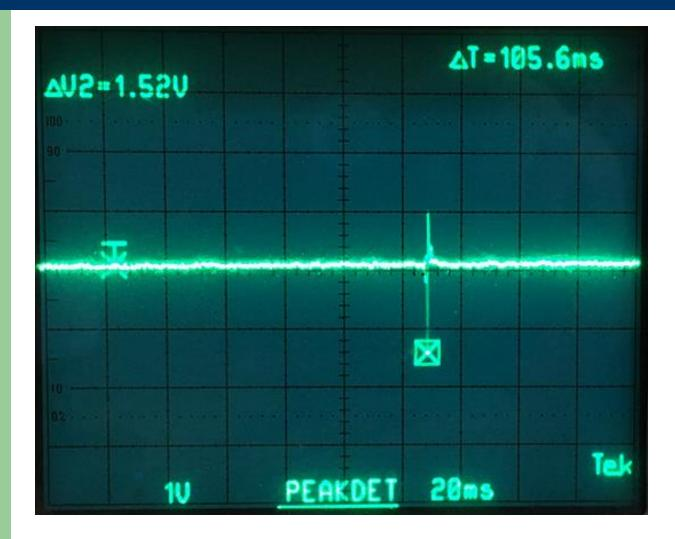
Latency of analog & SDR radios is all over the map from 2ms to 170ms.
