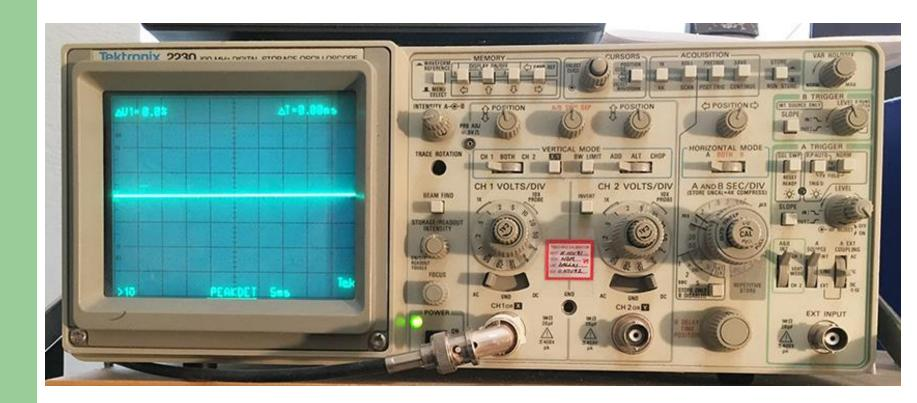
Set key down carrier to slightly over 6 divisions on scope. When speaking don't exceed 6 divisions = No Flat-topping ! Measured with \$100 Tektronix
