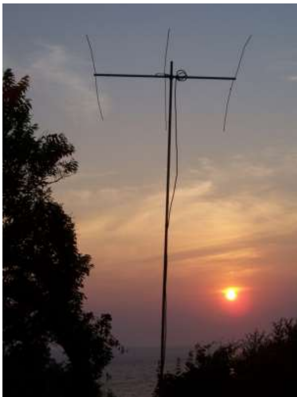
Three element Six Meter Yagi at Field Day site located in Eastern Long Island
