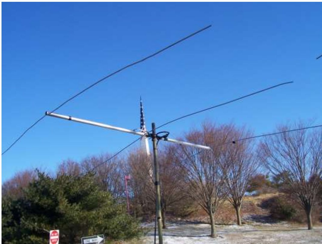
Three element Six Meter Yagi at a portable location for the January VHF Contest on hill 250 feet ASL in Central Long Island. Beam is mounted on pole, up 10 feet.
